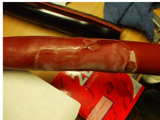
The replaced PD joint was dissected to check the position and level of PD erosion
